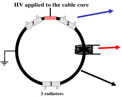
3 thermal diffusers to observe the homogeneity of the dielectric behavior of the insulator (OCT)
