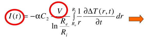
TSM current directly proportional to applied voltage
